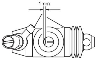
**Idle / Stop Screws** - Used for adjusting Idle: Set for 1/16th inch/1mm gap to start new engines. You can open more for higher idle.
