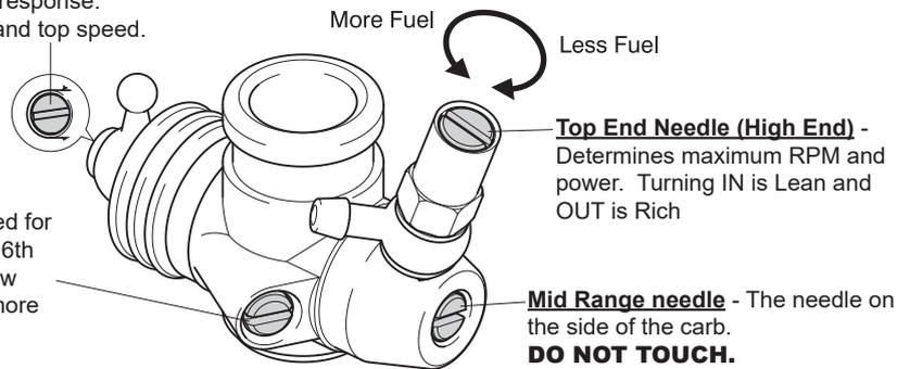
**Top End Needle (High End)** - Determines maximum RPM and power. Turning IN is Lean and OUT is Rich
